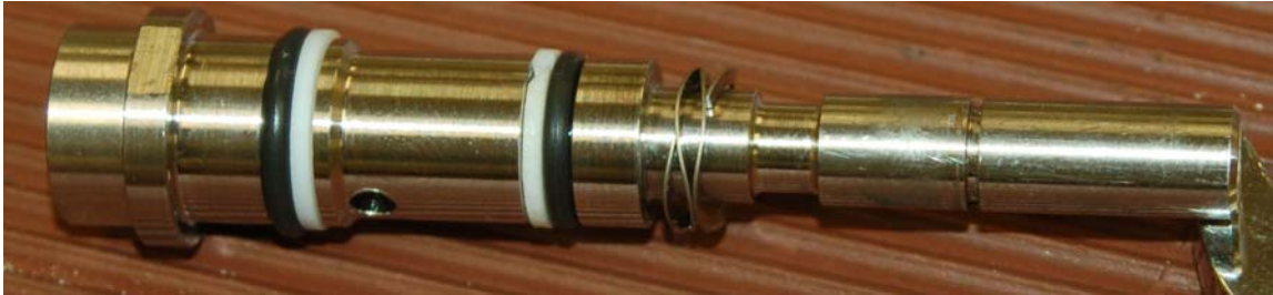
Step 6 Install Wave Spring, P/N 71003395 on Seat Holder, P/N 21457.
