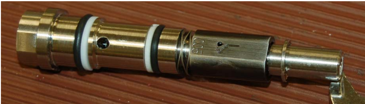
Step 7 Install Gate, P/N 22567 Install Retainer Washer, P/N 21461 on Seat Holder, P/N 21457
