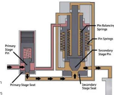
Gas charged first stage enacting when inlet pressure falls below gas charge
