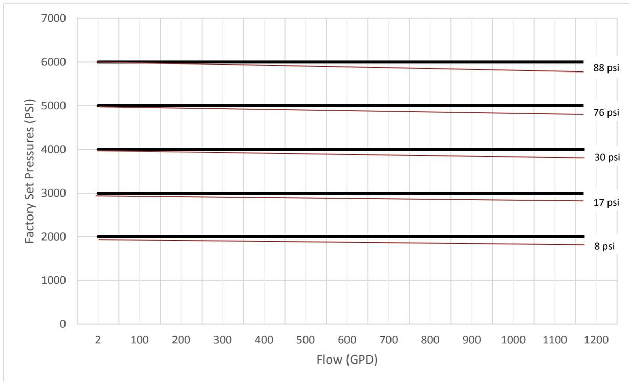
Performance characteristic of the Subsea BPR Set Pressure based on increase in flow
