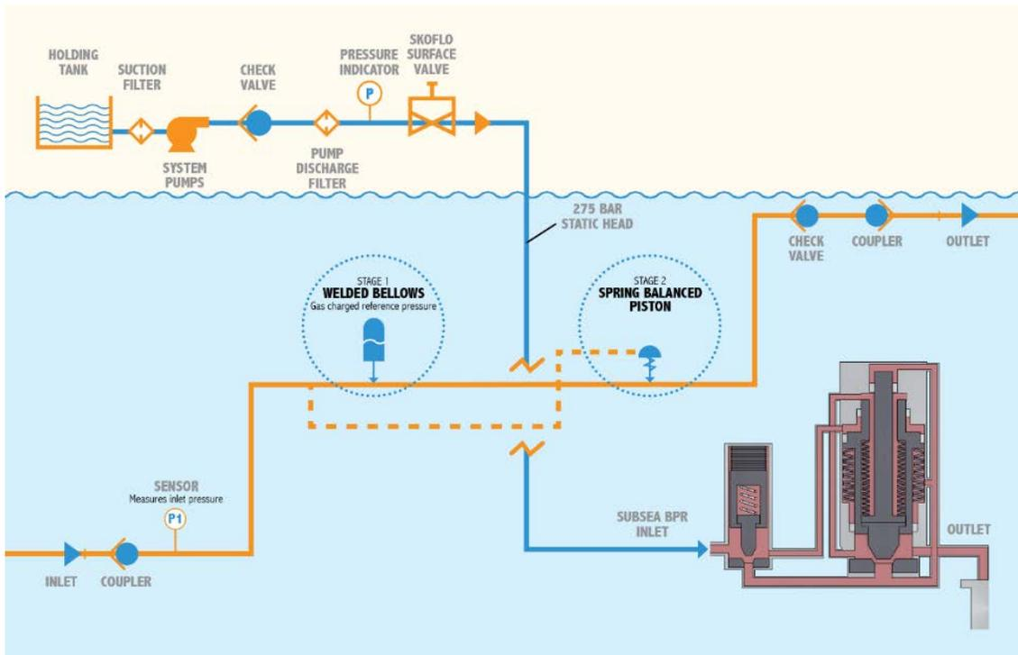
Figure 1.4 Subsea BPR P&ID (orange) and Chemical Injection Field Architecture Graphic
