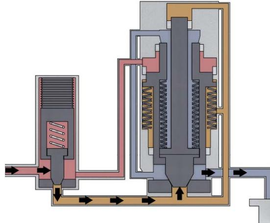
Figure 1.6: Second Stage minimizes cavitation and maximizes debris tolerance
