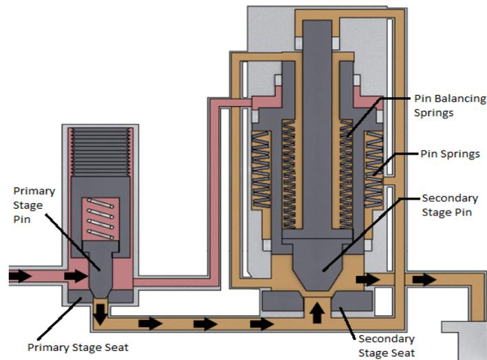
Figure 1.5: **First Stage** – A gas charge reference pressure activates a valve trim allowing the device to only regulate when the injection pressure falls below a set reference pressure. Otherwise, the device remains in the idle stage, which is simply a fixed orifice.
