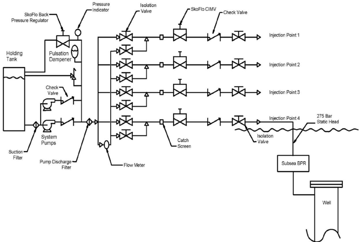
Figure 1.2 – Chemical Injection System Field Architecture
