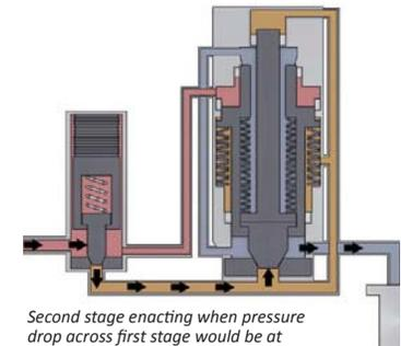
Second stage enacting when pressure drop across first stage would be at risk of cavitation damage
