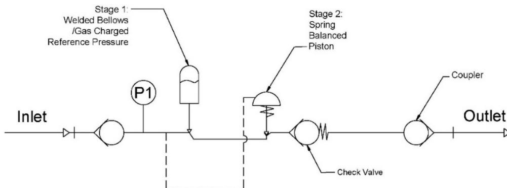
Figure 1.3 Subsea BPR P&ID
