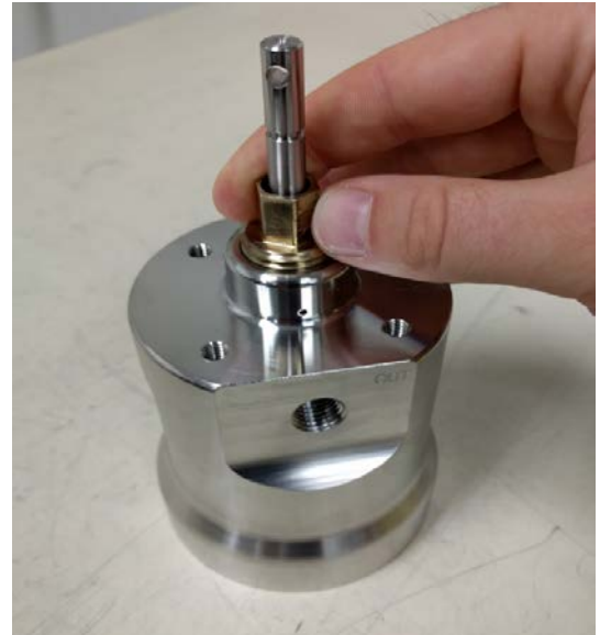
Figure 12 – Pressing Stem Seal into Groove
