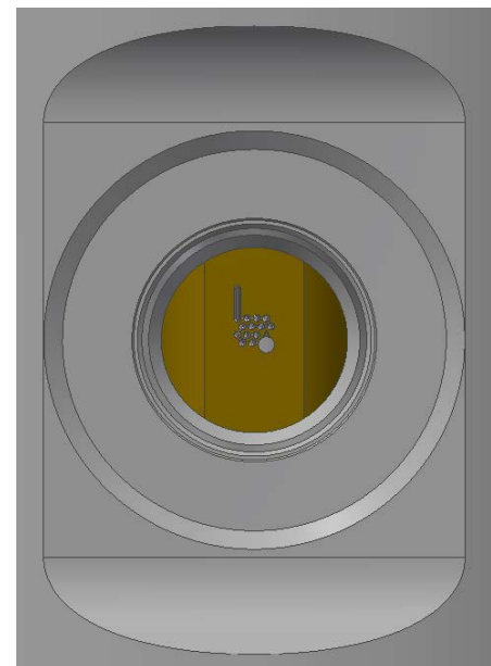
Figure 7 – Gate View Through Gate Pad Hole
