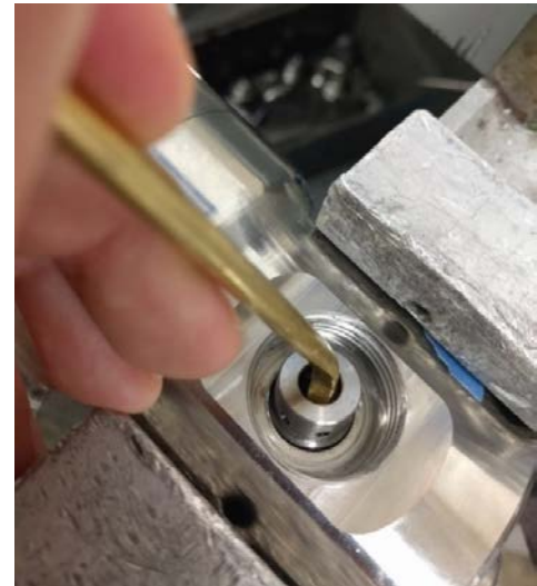
Figure 3 – Gate Pad Assembly Removal
