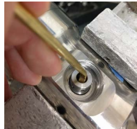
Figure 4 – Gate Pad Assembly Removal
