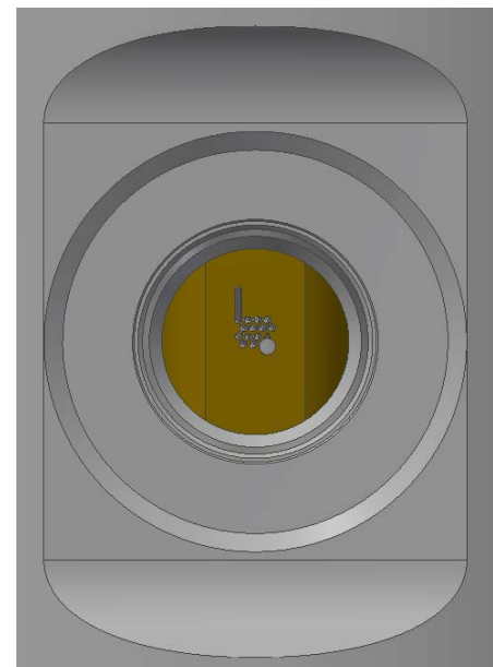
Figure 7 – Gate View Through Gate Pad Hole
