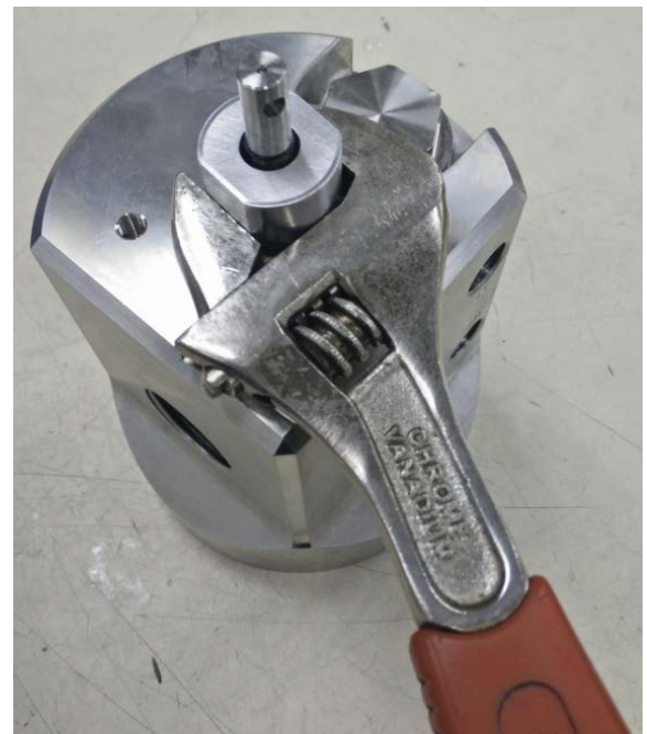
Figure 13 – Pressing Stem Seal into Groove
