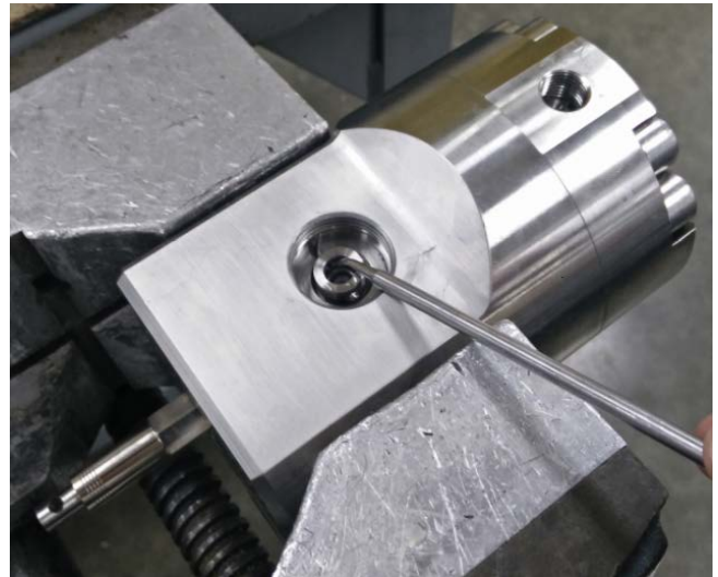
Figure 3 – Gate Pad Assembly Removal
