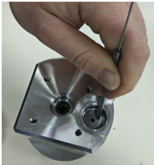
Figure 18 – Installing HPS Seat
