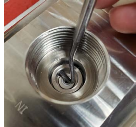
Figure 3 – Gate Pad Assembly Removal
