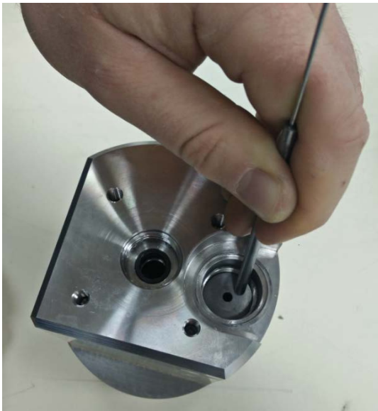
Figure 21– Installing HPS Seat
