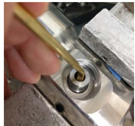
Figure 4 – Gate Pad Assembly Removal
